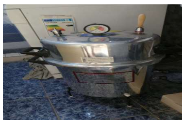
Larger 29L pressure cooker type autoclave
